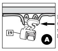
Insert one "arm" of clip into ram as shown. Twist "body" of clip slightly so that second "arm" slides over the top of the first "arm" as shown.
